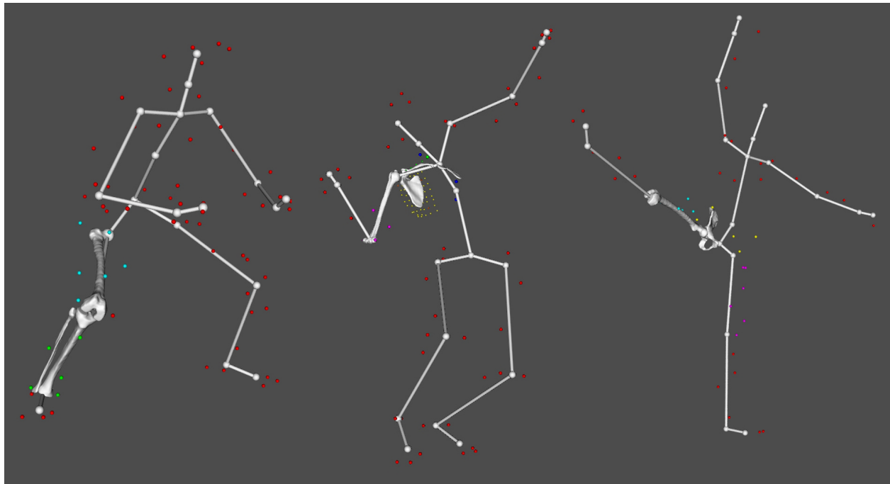
Figure 1.8: Computed postures for the knee, shoulder complex and hip obtained with the developed kinematic models: side step (left), tennis serve (middle) and dancing movement (right). Additional markers placed on the rest of the body and a virtual skeleton are also used to visualize the motion as a whole.
